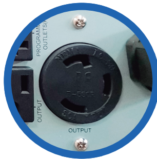
Output terminal NEMA L5-30R
