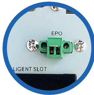
Emergency Power Off (EPO)
