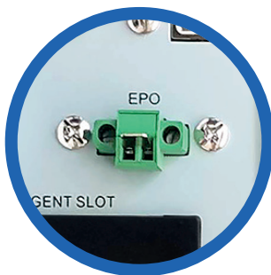
Emergency Power Off (EPO)
